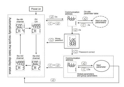
parameter setting mode, long pressing the Shift Key will return to the previous parameter. If the Set Key is pressed simultaneously, the user can exit the parameter setting mode immediately.
